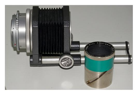
I used a M42 bellow from NOVOFLEX for M39 lenses. It is possible to focus the lens also at infinity. One excellent detail is that the lens has a "built in lens hood.
